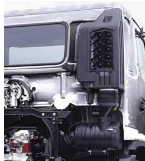
Larger air intake duct
